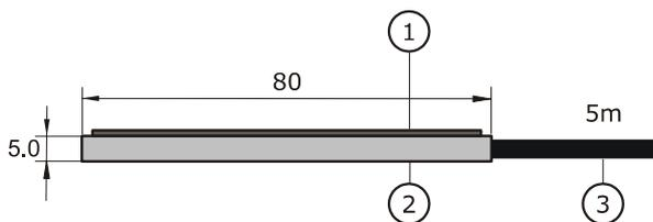
Figure 3 HFP01SC dimensions in mm: heater (1) heat flux sensor body (2), cable (3)
