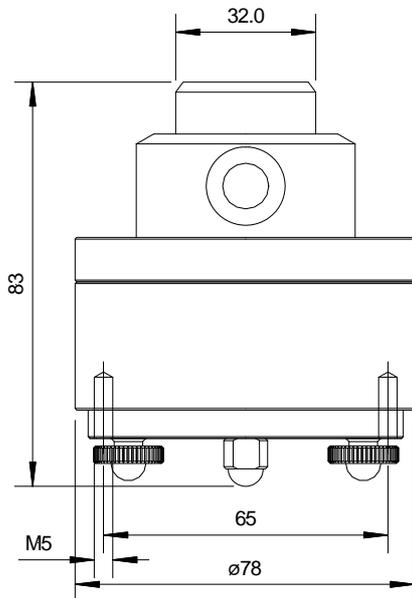
Figure 1 IR02-TR dimensions. Standard cable length is 5 m. Cable can be installed / replaced by the user.
