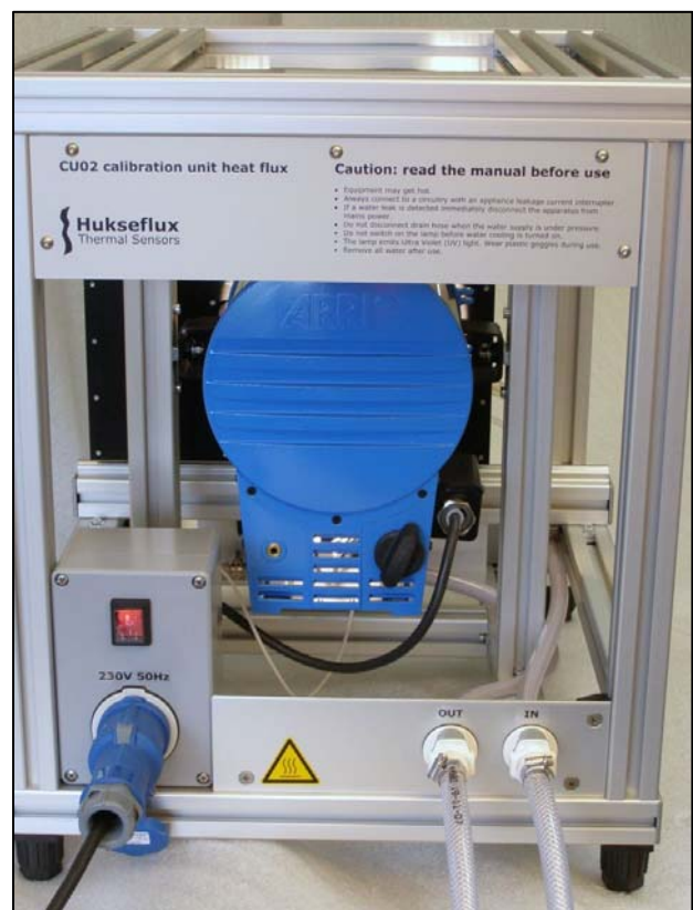
Figure 4: Picture of calibration unit CU02, showing water supply (in / out), power supply and heat source (1250 Watt lamp, housing in blue). At the background the water-cooled plate on which the sensors are mounted, is visible.
