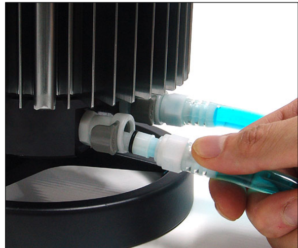
Figure 3: coupling of cooling tubes to the reserator
