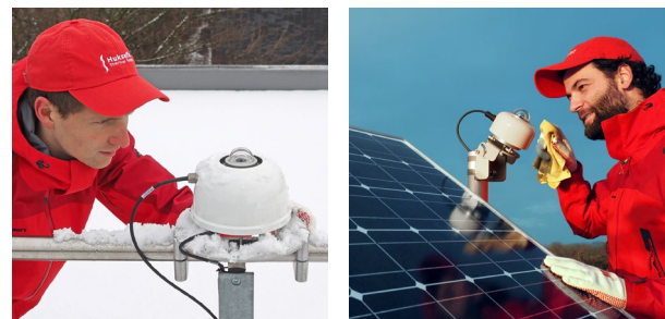
Figure 2 Left: a horizontally aligned pyranometer measuring the global horizontal irradiance (GHI) and right: a tilted pyranometer measuring a global tilted irradiance (GTI).
