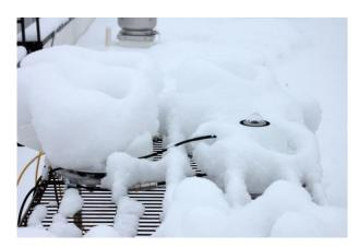
**Figure 5** Does ventilation work to remove snow? Not reliably: this photo shows 3 ventilation units in FEB 2014 in Logan UT, USA powder snow. Only 1 of the 3 pyranometers, the one at the right (SR20 with VU01), is visible. The other 2 are still covered in snow. Photo courtesy of Apogee Instruments Inc.
