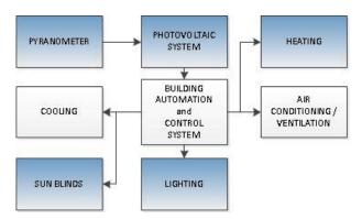
Figure 3 BACS with integrated pyranometer
