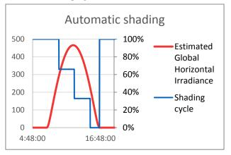
Figure 4 example of an automated shading strategy
