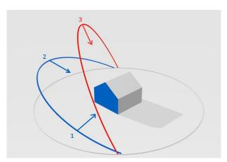
**Figure 2** incidence angles change during day and season. During morning in winter (1), the indicated façade receives a lot of sun. In the afternoon this is greatly reduced (2). In summer, much more light is reflected and the roof will receive more sun (3).
