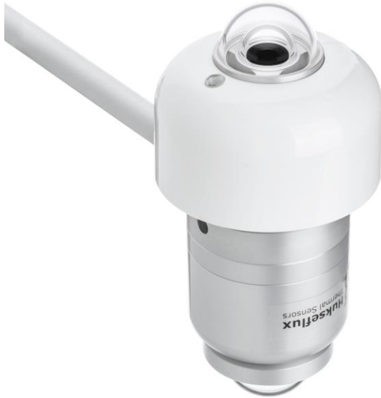
Figure 0.5 The end result using AMF03 and two SR30-D1 pyranometers: an SRA30-D1 albedometer ready for measuring
