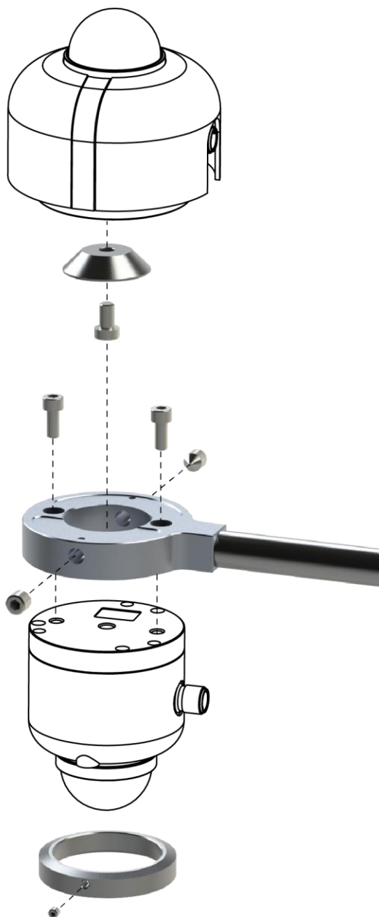
Figure 3.3.1 AMF03 with 2 x SR30 / SR15, mounting and fixation steps 1 – 7
