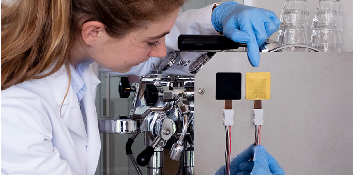
Figure 0.2 Working with BLK - GLD stickers: measuring the radiative and convective heat fluxes around an espresso machine.
