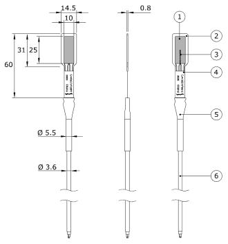
**Figure 4** FHF03 heat flux sensor: (1) sensing area with thermal spreader, (2) passive guard, (3) type T thermocouple, (4) sticker showing serial number and sensitivity, (5) strain relief, (6) cable, standard length is 2 m. Dimensions in  $\times$  10<sup>-3</sup> m.
