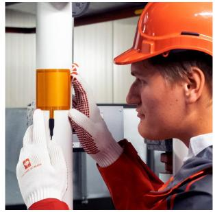
**Figure 2** FHF05-85X85 being installed to measure heat flux on a pipe
