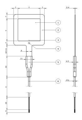
**Figure 4** FHF05-10X10, 50X50 or 85X85 heat flux sensor: (1) sensing area with thermal spreaders, (2) passive guard, (3) type T thermocouple, (4) dot indicating front side, (5) connection block, (6) cable, standard length C is 2 m. The size of Y can be 8, 36 or 70. All dimensions in  $\times$  10<sup>-3</sup> m.
