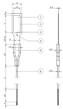
**Figure 5** FHF05-15X30 or 15X85 heat flux sensor: (1) sensing area with thermal spreaders, (2) passive guard, (3) type T thermocouple, (4) dot indicating front side, (5) connection block, (6) cable, standard length is 2 m. The size of Y can be 27 or 70. All dimensions in  $\times$  10<sup>-3</sup> m.
