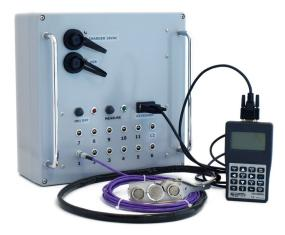
**Figure 4** the ALUSYS measuring system, for trend - monitoring and comparative surveys of heat fluxes and surface temperature on industrial installations.
