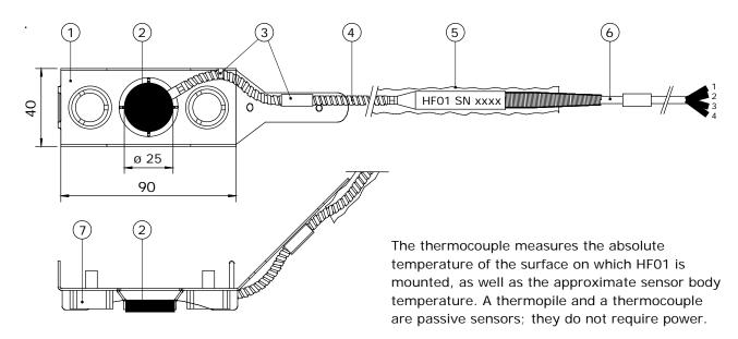
**Figure 2** heat flux sensor model HF01 with optional frame with magnets (2), connected to a high-temperature metal sheathed cable with interlocked spiral stainless steel armour (4) and low-temperature extension cable (6). The frame (1) with magnets (7) is an option intended for temporary mounting on carbon steel walls. It is provided with a cable strain relief (3). The armour may be electrically insulated by a silicone sleeve (5). Dimensions are in x 10<sup>-3</sup> m.
