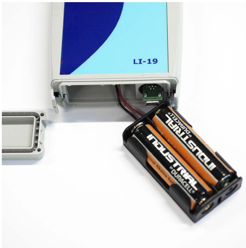
Figure 5.3.1 Battery replacement of LI19
