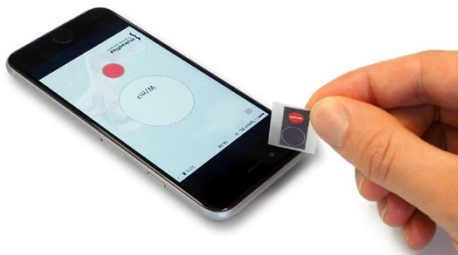
Figure 0.1 Cut diffusor and stick it on tape
