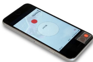
Figure 0.2 Cover camera lens with diffusor
