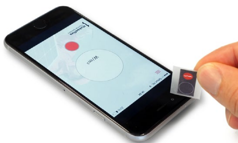
Figure 1.4.1 Stick diffusor on tape
