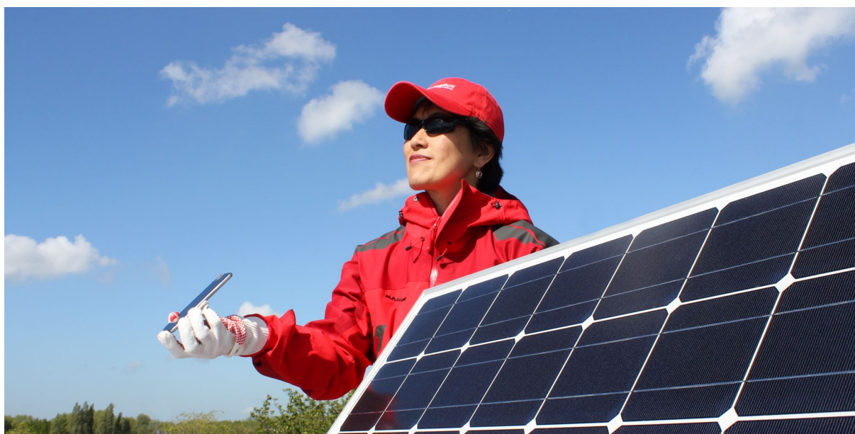
Figure 3.3.1 Alternative measurement measuring plane-of-array (tilted)
