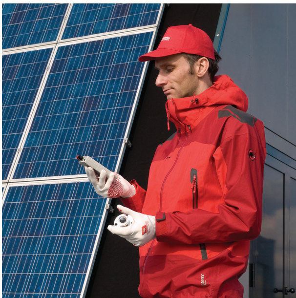
Figure 4 LI19 used with a pyranometer in a field measurement campaign
