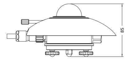
**Figure 3.2.1** Dimensions of SR20 in  $\times$  10<sup>-3</sup> m.
