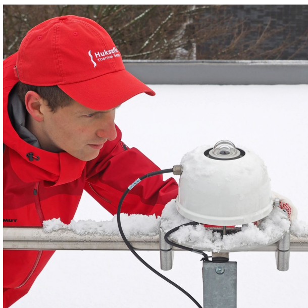
Figure 2 SR22 sensor combined with VU01 ventilation unit.
