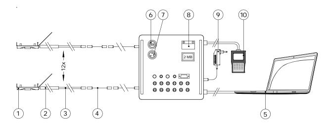
**Figure 2** the ALUSYS measuring system; (1) HF01 heat flux sensor (with magnet frame), (4) low temperature extension cables with 2 connectors, (5) PC or laptop (not part of the system). On or inside the MCU: (6) chassis connector for PC connection via USB, (8) rechargeable battery and system memory. Outside the MCU: (9) adapter (100 - 240 VAC) and
