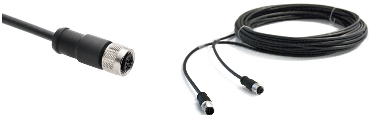
Figure 0.3 On the left the DR30 cable with M12-A female connector on sensor end, pigtails of 0.15 m and conductors with ferrules. Its length is 5 metres standard and available in 10 and 20 metres too. On the right the optional Hukseflux extension cable with connector pairs, with male and female M12-A connectors, available in 20 metres.
