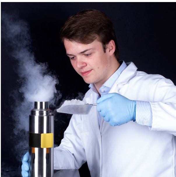
Figure 7 Model FHF05-50X50 with BLK and GLD stickers for measuring insulation losses of a thermos.
