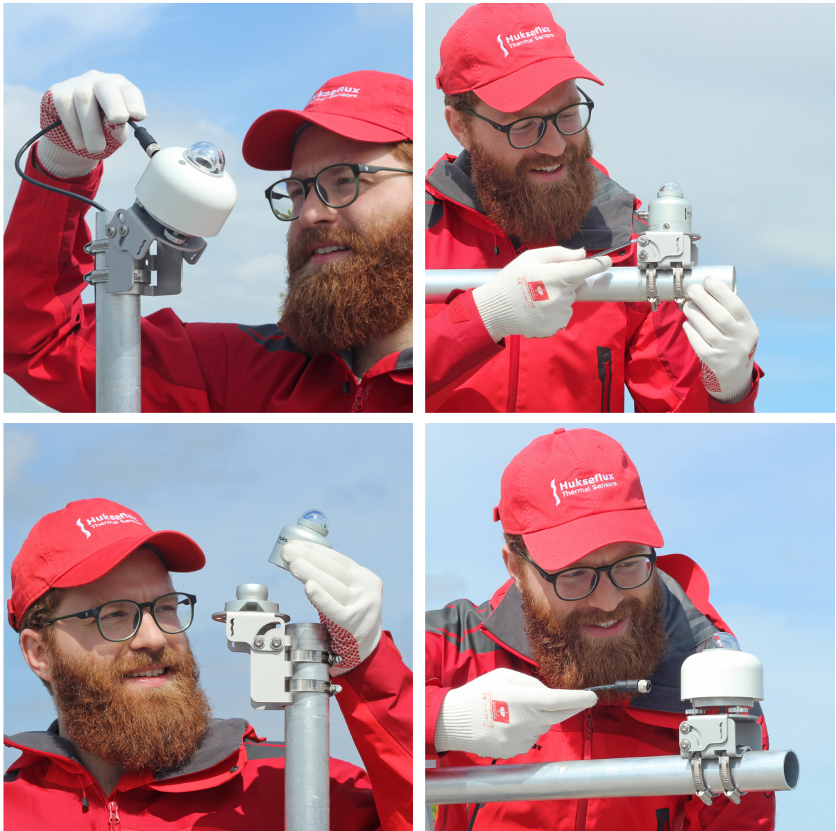
Figure 0.4 Hukseflux pyranometers with PMF01 pyranometer mounting fixtures on a horizontal crossarm and on a vertical mast, being installed both in Plane of Array (tilted) and horizontally. The versatile PMF01 allows for mounting on a surface, using bolts, as well
