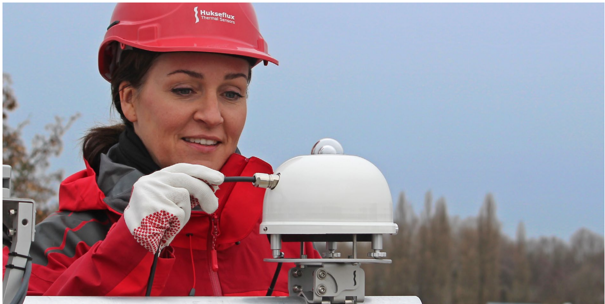
Figure 0.5 VMA01 is a mounting adapter allowing installations on PMF01 of the small footprint VU01 ventilation unit with a suitable Hukseflux pyranometer, horizontally or tilted
