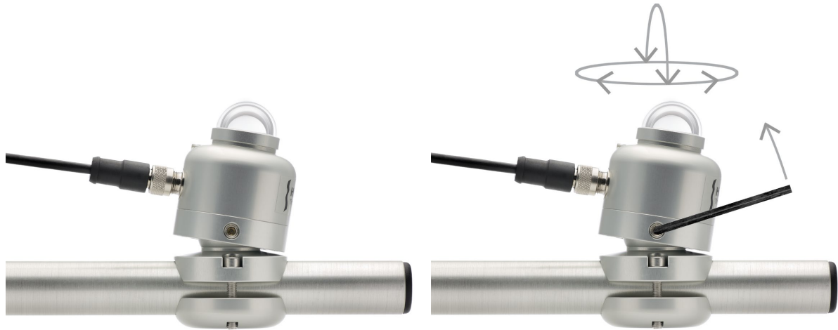
1) judge bubble level and cable orientation 2) loosen set screw to tilt and rotate SR05
