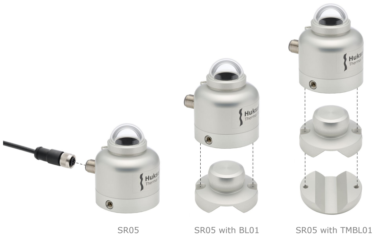
Figure 5.2.1 From left to right: SR05 in its standard configuration with 3 metre cable; with optional ball levelling for easy mounting and levelling on a (non-)horizontal surface; with optional ball levelling and tube mount for easy installation on a 25 to 40 mm diameter tube. Mounting bolts are included with the ball levelling and / or tube mount.
