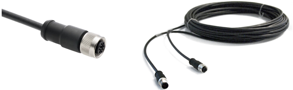
Figure 0.4 On the left the SR15-A1 cable with M12-A female connector on sensor end, stripped over 0.15 m and conductors with ferrules. Its length is 5 metres standard and available in 10 and 20 metres too. On the right the optional Hukseflux extension cable with connector pairs, with male and female M12-A connectors, available in 20 metres
