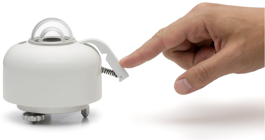
Figure 5.2.2 Installation of SR15-A1's sun screen
