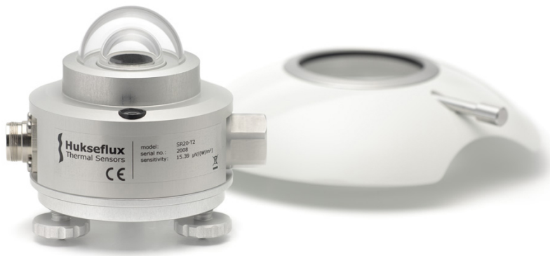
Figure 0.1 SR20 secondary standard pyranometer with its sun screen removed
