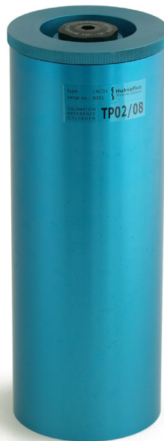
Figure 0.6 A CRC01 calibration reference cylinder containing a polymethylmethacrylate reference material for calibrating TP02 and TP08
